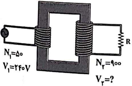
$\frac{V_2}{V_1} = \frac{N_2}{N_1} \rightarrow \frac{V_2}{240} = \frac{900}{50} \rightarrow V_2 = 4320 V$
