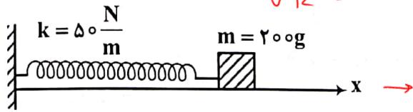
$$T = 2\pi \sqrt{\frac{m}{k}} = 2\pi \sqrt{\frac{0.2}{50}} = 2\pi \sqrt{\frac{2}{500}} = 2\pi \sqrt{\frac{1}{250}} = \frac{2\pi}{\sqrt{250}} = \frac{2\pi}{5\sqrt{10}} \approx 0.5 \text{ s} \quad (\pi = \sqrt{10})$$
